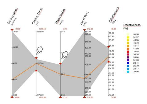
Virtual experimentation for continuous casting to establish robust process windows
