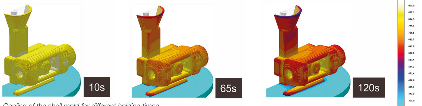
Cooling of the shell mold for different holding times
