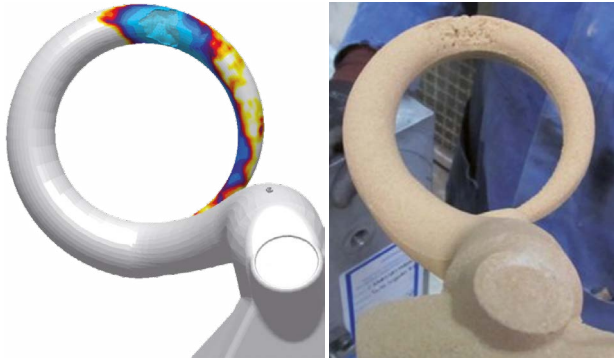
Identifying and evaluating defect root causes
